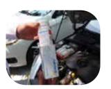
When the sample container is full, it is disconnected from the pump and the lid is immediately attached.
