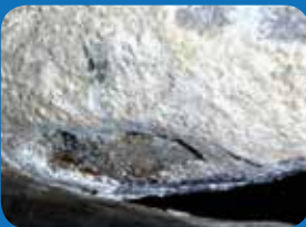
Calcification in the cylinder liner arising from the use of very hard water
