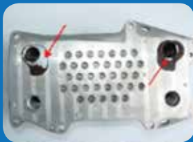
Cavitations in oil cooler due to the use of unsuitable antifreeze
